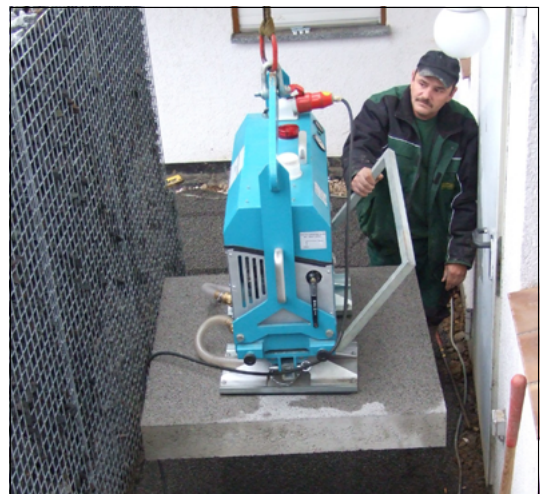
Kappa Levator with electric motor, carrying capacity 800 kg.
