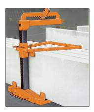
Off loading yoke for panels AbBü 3.4 for the transport of vertically positioned panels and packages.
